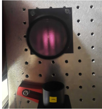
Figure 3.12: Examination of the beam collimation after the second achromatic lens with a shear plate interferometer. The alignment of the red stripes inside the interferometer parallel to the optical axis confirms that the beam is collimated again after being decollimated by the first achromatic lens of the setup in Fig. 3.11.
