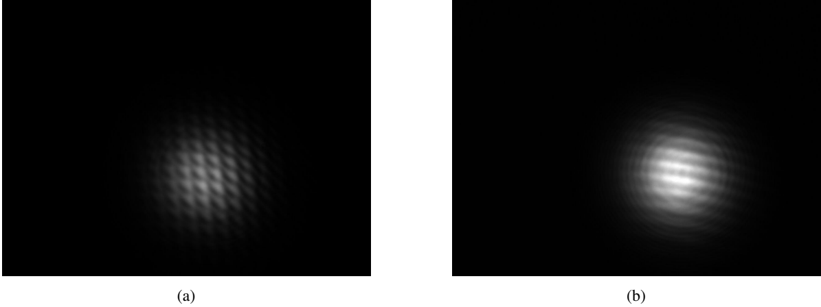
Figure 3.4: Image of the collimated probe laser beam taken with the Thorlabs CS165MU/M camera. (a) Due to reflections at the glass pane protecting the sensor and within the silicon sensor itself a pattern of light and dark triangles can be observed. (b) After removing the glass pane, only the interference due to the reflections in the sensor can be observed.
