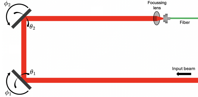
Figure 2.1: Sketch of a simple fiber coupling setup with four labeled angular displacements of the mirrors. The pitch angles are \theta_1 and \theta_2 , and the yaw angles are \phi_1 and \phi_2 . The mirrors guide the input beam towards the focussing lens, which focuses the beam to the size of the fiber core in order to collect the laser light with the fiber. Image modified from [13].
